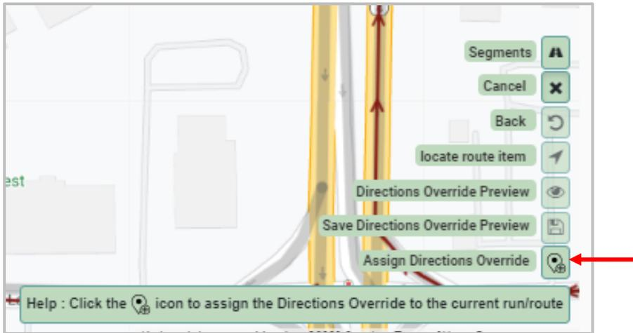
Selecting the “Assign Directions Override” tool will populate the following screen where the router can then opt to “Assign the DO to [the] currently selected run cover”.
