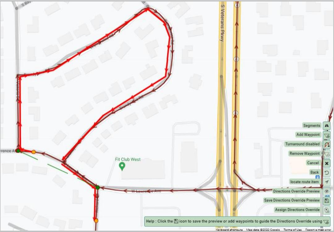
The bold red line is what the system has determined the new path to be, so in some cases there is a need to use waypoint tools to help guide the Direction Override.
